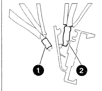
Checking control relay and startingmotor solenoid
